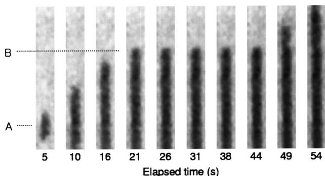
FIG. 3. Time-resolved domain images of a magnetic strip with a constant time step. The strength of the magnetic field was 355 Oe, smaller than the coercive field of 550 Oe. The domain wall propagation in a constant speed and the pinning are clearly seen from the figure.
