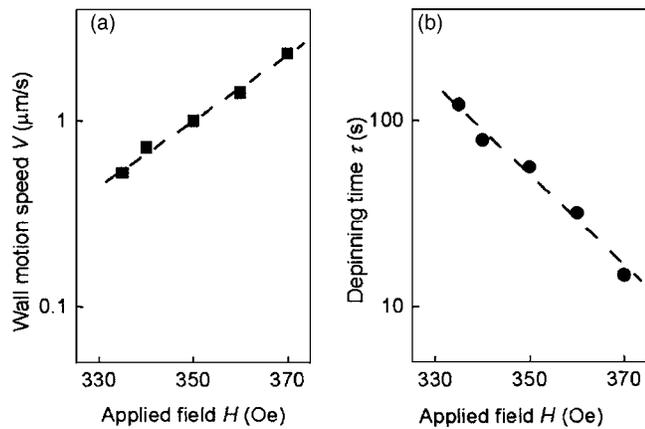
FIG. 5. (a) The magnetic field dependence of the wall propagation speed. The dashed line shows the best fit using Eq. (1). (b) The wall pinning time of the pinning site located at “B” in Fig. 3, with respect to the strength of an applied magnetic field. The dashed line shows the best fit using Eq. (2).
