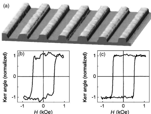
FIG. 1. (a) Topological image taken by an atomic force microscope. The width of the strips was  $2 \mu\text{m}$  with a  $4 \mu\text{m}$  periodicity. (b) Local magnetic hysteresis loop measured on the strip. (c) Magnetic hysteresis loop measured on the unpatterned area of the sample.
