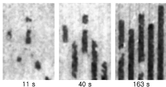
FIG. 2. Time-resolved domain images of periodic magnetic strips under a constant magnetic field. The reversed domains were formed in the beginning and then propagated along the strips in time.
