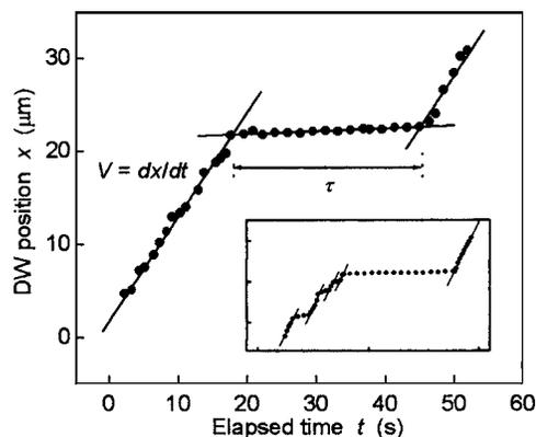
FIG. 4. The position of the domain wall front  $x$  with respect to the elapsed time  $t$ , measured from the images shown in Fig. 3. The linear fitting lines guide the wall propagation. The inset shows another stepwise process seen from other strips.
