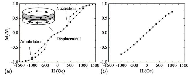
FIG. 3. Simulated hysteresis curve for (a) 500-nm-diameter, 20-nm-thick Py layers separated by a 1-nm-thick nonmagnetic spacer with bilinear exchange coupling of  $-250$  Oe. (c) Simulated in-plane minor hysteresis loop for 500-nm-diameter, 40-nm-thick Py layers separated by a 1-nm-thick nonmagnetic spacer, neglecting bilinear exchange coupling. This hysteresis-free response corresponds to vortex displacement.
