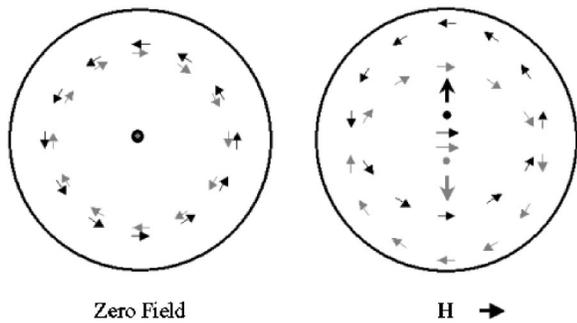
FIG. 4. The vortex core positions and directions of rotation are illustrated schematically for the top and bottom disks in black and gray, respectively, corresponding to those in Fig. 3.
