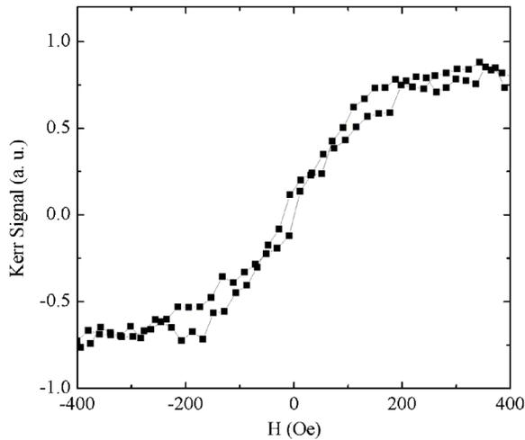
FIG. 2. In-plane MOKE hysteresis curves for 20 nm thick, 2  $\mu\text{m}$  in diameter Py disks separated by 1 nm of Cu (mid-sized disks in Fig. 1).
