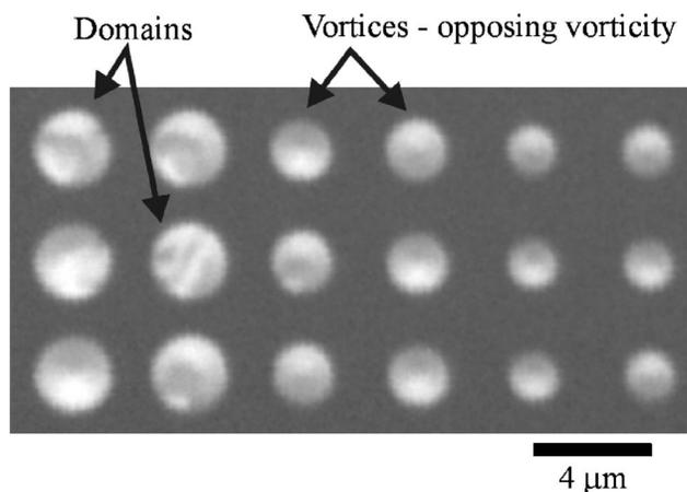
FIG. 1. PEEM images showing the in-plane magnetization state of the top disk for Py/Cu/Py layers (diameters of 1.2–2.5  $\mu\text{m}$ ), where the Py layers are 20 nm thick and the Cu is 1 nm. The grayscale map is proportional to the magnetization alignment with the in-plane direction of incidence of the x rays (long axis of the array) where white and black represent saturation in opposing directions.
