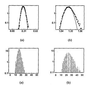
Fig. 1. Distribution density of the local coercivity of the 500-Å  $Si_3N_4/400$ -Å  $(Co_{72} Cr_{18})_{100-x} Pt_x/1100$ -Å Ti alloy films with (a) x=6 at.%, (b) x=28 at.%.
