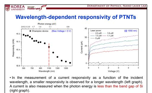
• This wavelength-dependent current generation can be understood by a broad range of energy levels for the trap states. The current is generated by photon triggering of the trapped electrons in the PSi segment.
