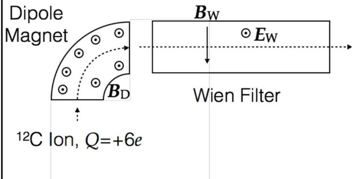
(a) [10 pts] Charged ions enter into the entrance of the dipole magnet. The ions are characterized by their charge  $Q$ , mass  $M$  and speed  $v$ . Find the necessary condition for some ions to exit the dipole magnet through the circular trajectory. The magnetic field of the magnet is  $B_D$ , and the radius of the curvature of the trajectory inside the magnet is  $\rho$ .
