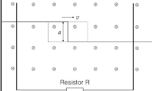
(a) [15 pts] The wave front (the position of the step) enters a region with uniform magnetic field  $B$ , as shown on the Figure. ( $B$  is applied 'upwards' on the paper.) Compute the electromotive force on the wire.
