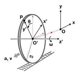
• (a) If we adopt the x-y frame centered on the initial position of the tire's center, this question may remind some students of Problem 10 in Homework #1 of Classical Mechanics 1 (2020). The point P's velocity measured in the x-y frame becomes  $\mathbf{v}_{\mathrm{f},P} = (-v - r_0\dot{\theta}\cos\theta)\,\hat{\mathbf{e}}_x - r_0\dot{\theta}\sin\theta\,\hat{\mathbf{e}}_y$
