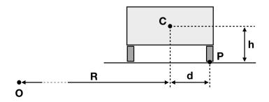
• (a) When the car is about to overturn, no normal or frictional force acts on the inner wheel. So, the normal force acting on P (see the figure) is  $N_P = mg$ , and the frictional force on P becomes the centripetal force,  $F_P = \frac{mv^2}{R}$ . One last condition to add is that there is no net torque about C, meaning  $F_Ph = N_Pd$ . Combining the equations, one arrives at  $\frac{mv^2h}{R} = mgd$ .
