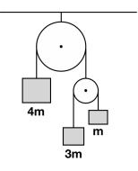
• (a)  $x_1$ : distance between the center of mass of the larger pulley (pulley 1) and 4m,  $x_2$ : distance between the center of mass of the smaller pulley (pulley 2) and 3m, then,  $4m\ddot{x}_1 + 3m(\ddot{x}_1 - \ddot{x}_2) + m(\ddot{x}_1 + \ddot{x}_2) = 0$  and  $-3m(\ddot{x}_1 - \ddot{x}_2) + m(\ddot{x}_1 + \ddot{x}_2) = 2mg$  (discussed in the class or in Example 7.8)
