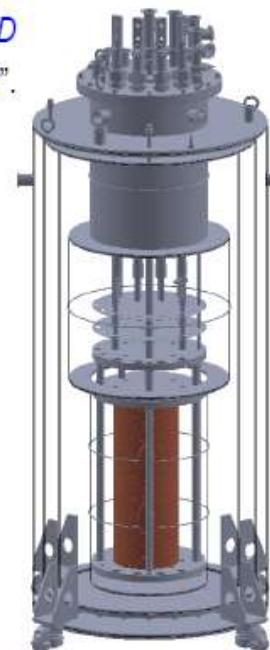
[35 T Magnet in the Existing Multi-Purpose Cryostat at KBSI](#)
