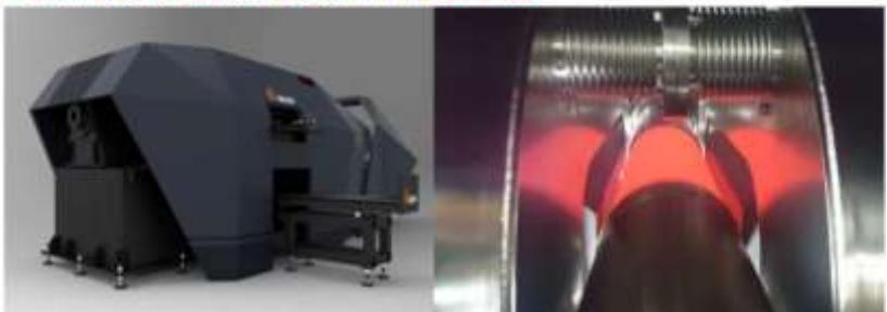
Real 3D design of the 300 kW superconducting induction heater
